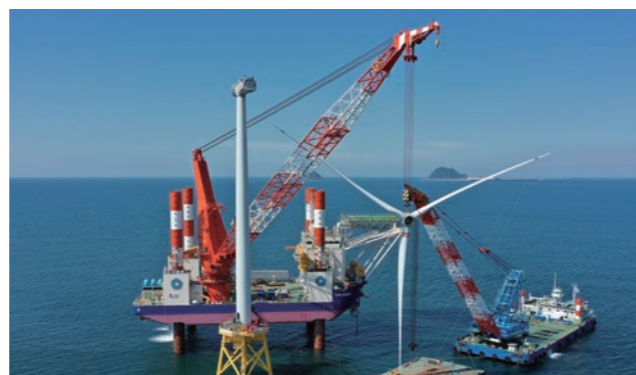
CP-8001 わが国初のSEP船(800t吊)
