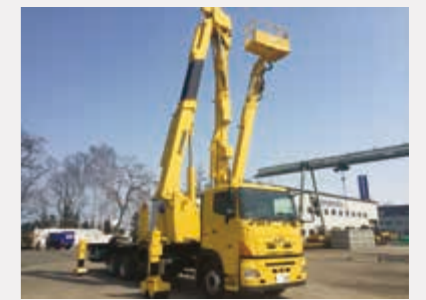
当社の橋梁点検車 Kanamoto Bridge Inspection Vehicle
