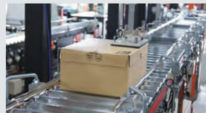
After packing, the two-dimensional code on the box is read and the corresponding invoice is affixed.
