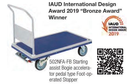
Pedal makes the truck easy to get moving from a static position
