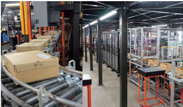
I-Pack® (high-speed automated packaging and shipping line) required for direct deliveries to users
